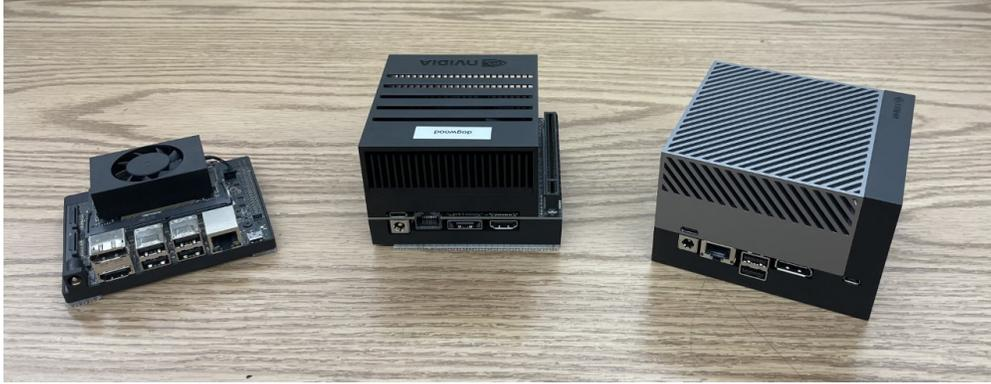
Figure 4.7: Here we can see, going from left to right, the Jetson Xavier NX, Jetson Xavier AGX, and the Jetson Xavier Orin. Each is powered by a variable output buck converter onboard the vehicle or the provided power supply which can be plugged into the wall.
