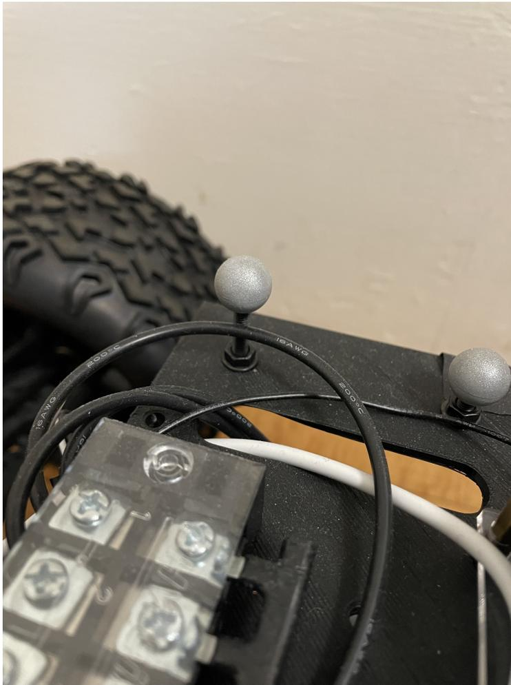
Figure 4.6: Here are two retroreflective markers which were placed on the second ART vehicle.
